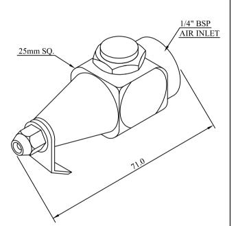
APPLICATION: For Blowing of dirt, dust, oil etc. from shop floor, surfaces, machine working area, deep holes, crevices, geometric patterns, etc. and any hard to reach places.
